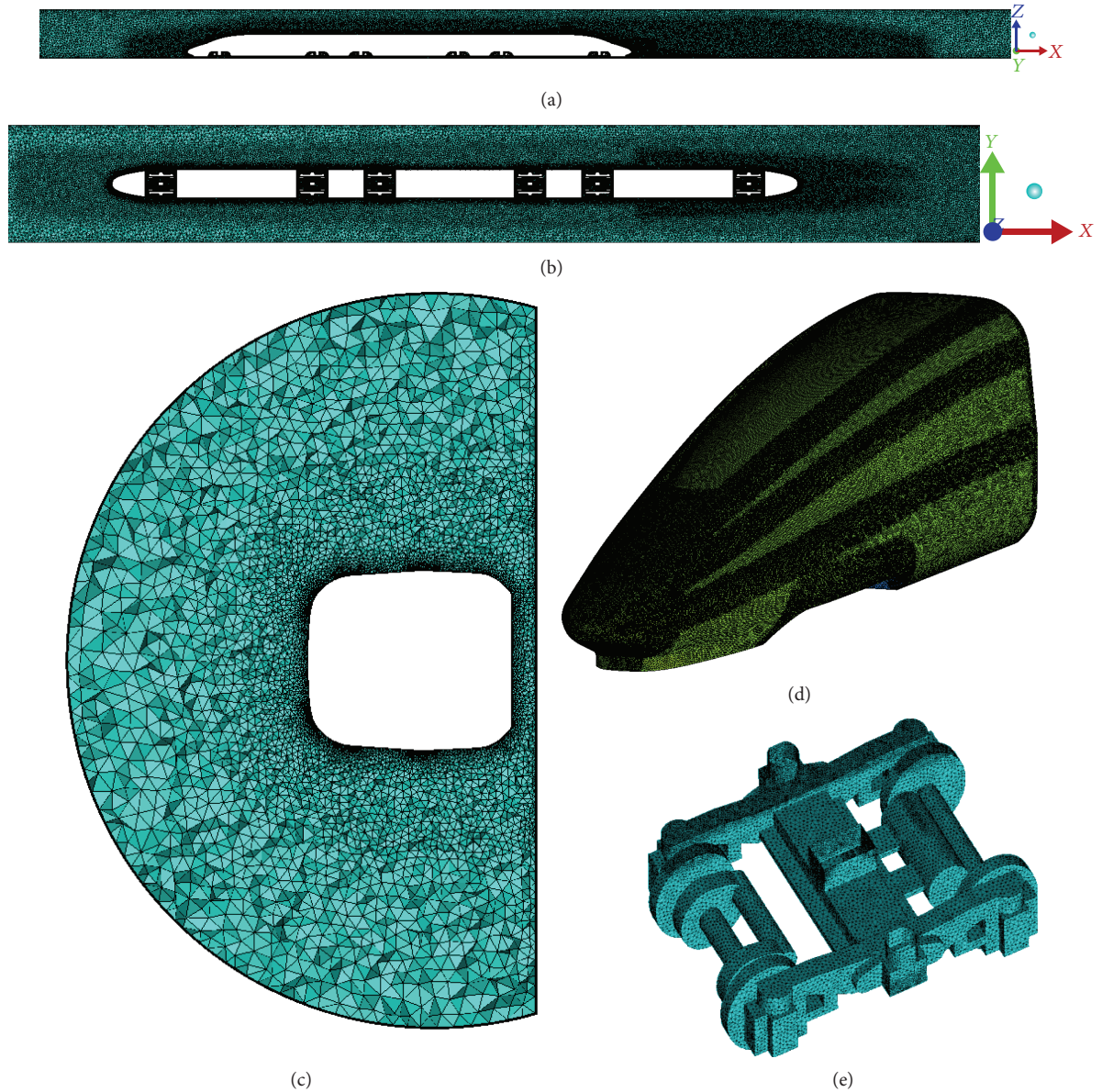
FIGURE 3: Mesh distribution: (a) longitudinal plane, (b) x - y plane with a height of 0.1 m from the ground, (c) cross section of the streamlined shoulder, (d) streamlined part, and (e) bogie.
